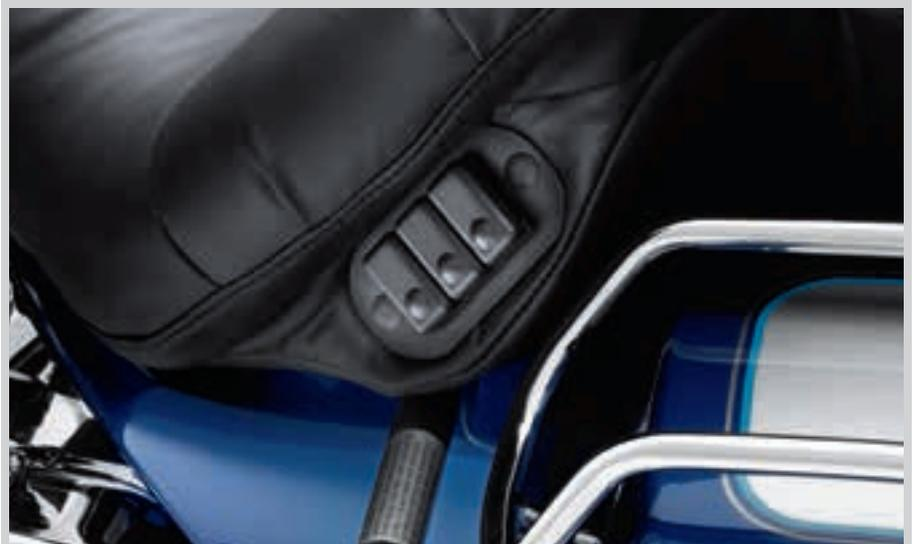
A. ROAD ZEPPELIN SITZE MIT EINSTELLBAREN LUFTPOLSTERN – BEDIENTAFEL
